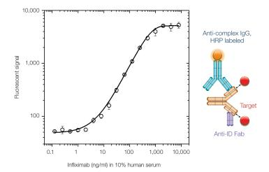
Anti-Infliximab Antibody, Type 2 (#HCA214) was used as the coating antibody (1.0 µg/ml) followed by infliximab spiked into 10% human serum as the antigen. Detection was performed by adding HRP conjugated Anti-Infliximab Antibody, Type 2 (#HCA216P, 2.0 µg/ml).
